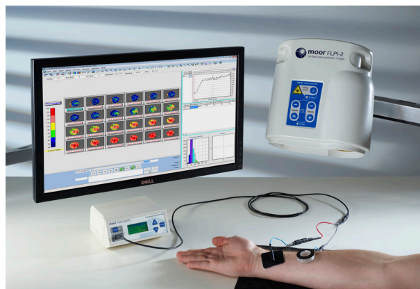
moorFLPI-2 and MIC2 – Experimental set-up displaying skin blood flow response to Acetylcholine.
