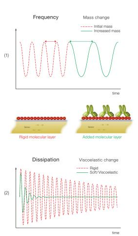
The Q-Sense E4 is a real-time analytical instrument for studies of molecular events occurring on surfaces. The E4 measures mass and viscoelastic properties of molecular layers as they build up or change on the sensor surface. Q-Sense E4 instruments play a key role in areas such as materials, protein and surfactant research.
