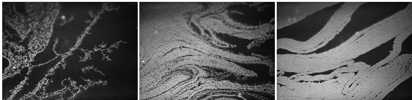
KSV NIMA MICROBAM IMAGES: STEARIC ACID MONOLAYER FORMATION DURING COMPRESSION
