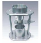
The manual ERWEKA SMG is the unit for the reproducible determination of apparent (bulk) density which can be used with all free falling powders or granules.
