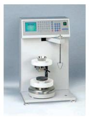
On the GT and GTL flow ability testers a special dynamic balance is integrated which allows the user to measure stable weight while the sample is falling on it.
