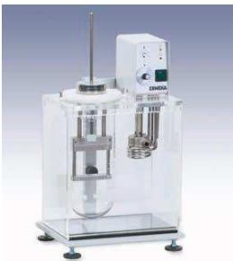
Suppository Hardness Tester, type SBT 2.
