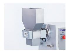
Dry granulator with two driven rollers running in opposing directions from the inside to the outside.
