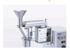
The CM is a product in feed system for application for development in pharmaceutical and food industry, which comminute powdery and free flowing products by a sieve with fixed maximum sizes of impurity-free granule (adjustable 0.3 – 3.0 mm; perforated round holes, grater holes or square holes).
