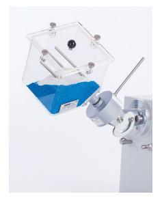
The Cube Mixer uses a tumbling motion to produce a homogenous blend within a short time. The mixing action is assisted by three stainless steel rods strategically positioned within the cube.
