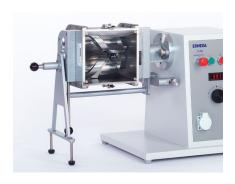
Laboratory kneader with stainless steel kneading vessel (5 liter volume, working capacity 65%) housing two z-shaped kneading blades running at different speed in opposing directions.
