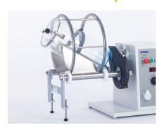
Drum hoop mixer with diagonal placement of the drum within the hoop. The rotation of the hoop itself produces a uniform, three-dimensional displacement of the material to be processed and hence a tumbling mixing action.
