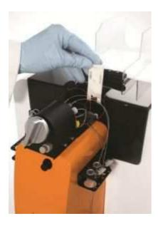
2) Insert sensor slide into the instrument
