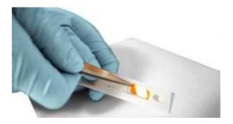
1) Insert sensor slide into a sensor-slide holder.
