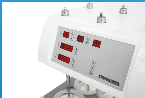
LED-display and symbol keypad for easy control
